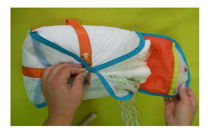
■ Use a pen like tool in order to keep the container from opening while packing the lines.
